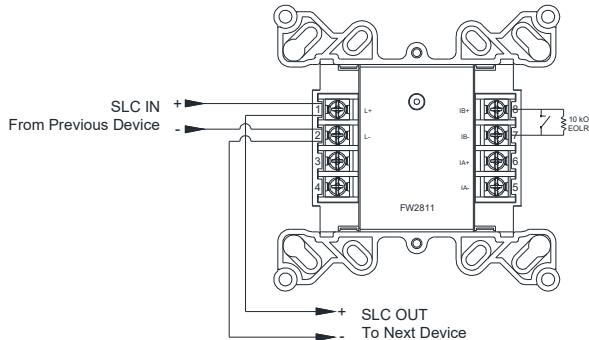
**Note:** check module installation instruction sheet for more installation and wiring options and details.
